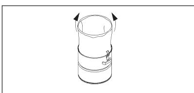
4. Reassemble the cyclonic separator and the bag support into the waste container ensuring all parts are clean and not damaged.
