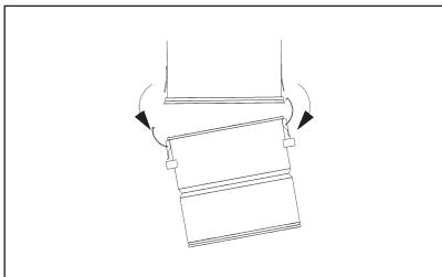
6. Re-connect the container with the machine being careful not to damage the seal edges which would cause a loss of suction (close both clamps together).
