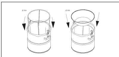
5. Carefully place the waste container up to the bottom of the machine in order to make a good seal.
