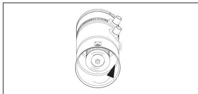
3. Extract the filter (for model: 45/2-3 also the metal grill) and proceed to clean it using a compressor, traditional vacuum or by a simple shaking motion, being careful not to damage it.
