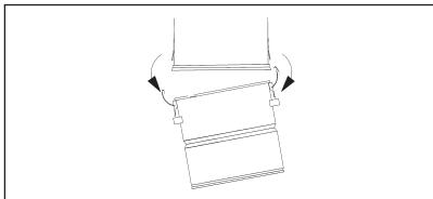
2. Remove the cyclonic separator and bag support frame
