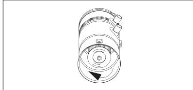
2. Rotate the finger grip anticlockwise until the filter can be removed.
