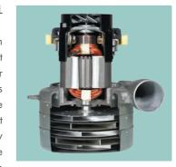
used in the aeronautics field, the carbon brushes are longer than the standard ones. It is well balanced in order to have high performances and to last longer than any other motors. The tangential motor used by Disan has separate cooling fans. The suction chamber is sealed, thereby protecting the electrics and exhausting any impurities to the outside. The electrical side with its own fan is self cooling and independent from the suction chamber.
